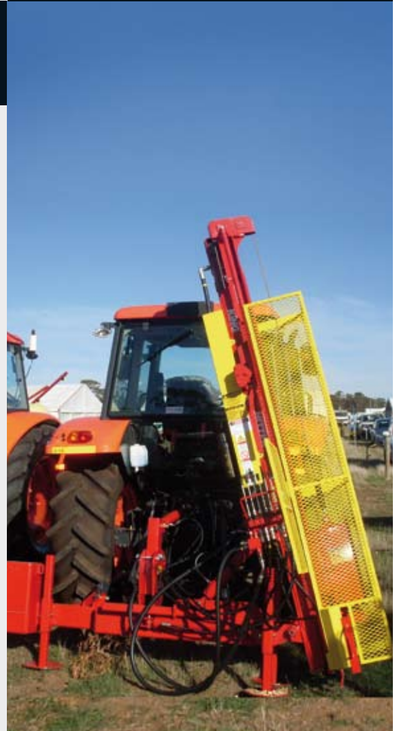
Series III Expander (Compulsory Safety Guards)
